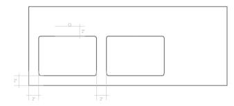
The minimum gap between a cutout and the edge of the slab must be at least 2". The size recommends distances greater than 2" when the kitchen design allows as it makes the countertop firmer.
